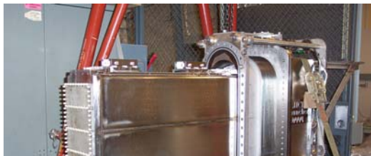
Figure 3.1.6: The forward wave guide assembly ready to be installed into the vacuum test stand.
