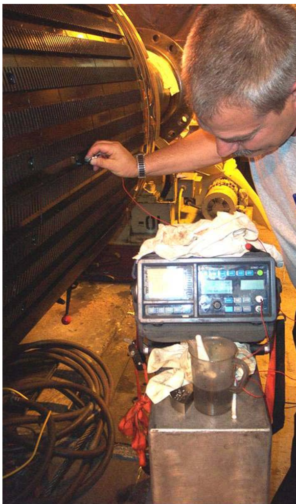
Figure 3.1.1: Detailed UT tests of critical alternator rotor locations have been performed.
