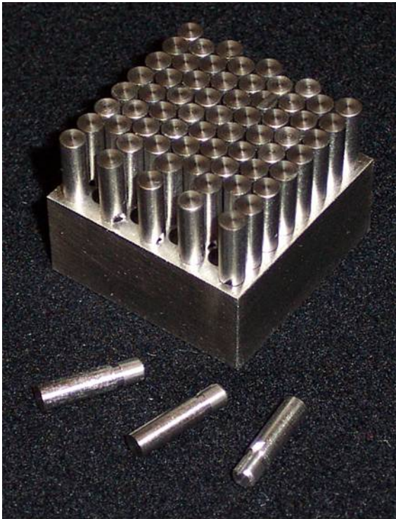
Figure 3.1.4: Prototype tungsten brush tile is shown together with three of the tungsten rods.
