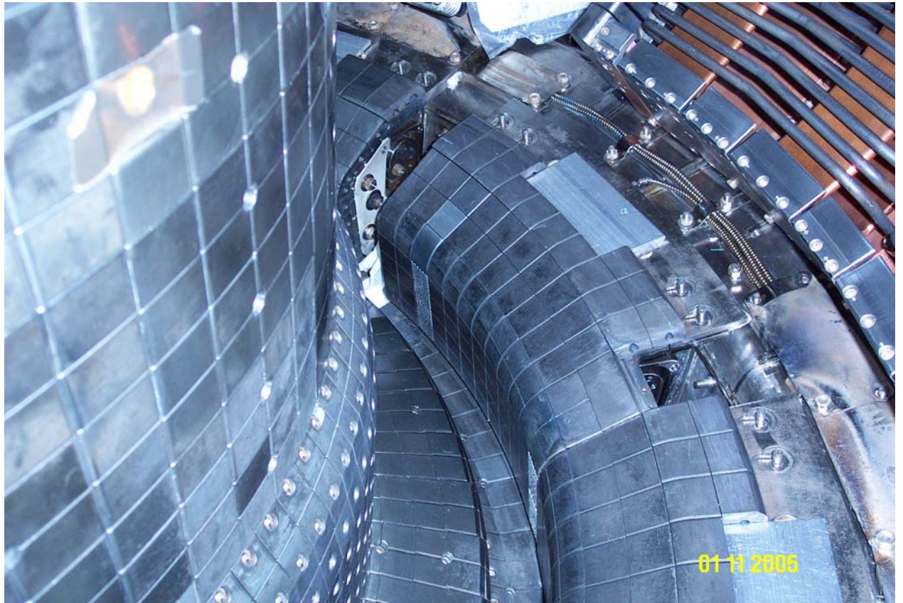
Figure 3.8: Tungsten brush tiles installed in C-Mod. Twelve tiles were installed at 3 toroidal locations (two locations shown).
