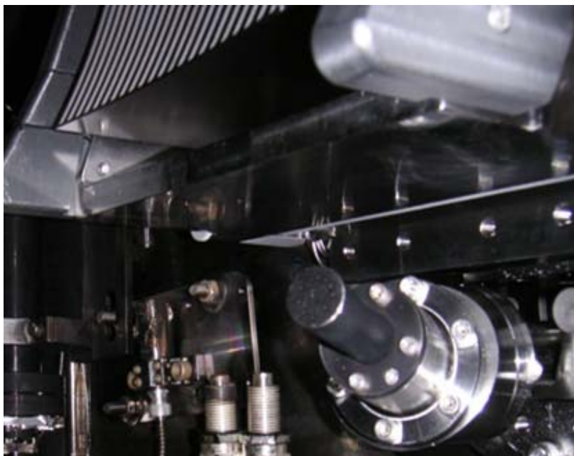
Figure 3.10: The tangential compact neutral particle analyzer (TCNPA) will measure the charge exchange neutrals from the ICRF produced ion tail.
