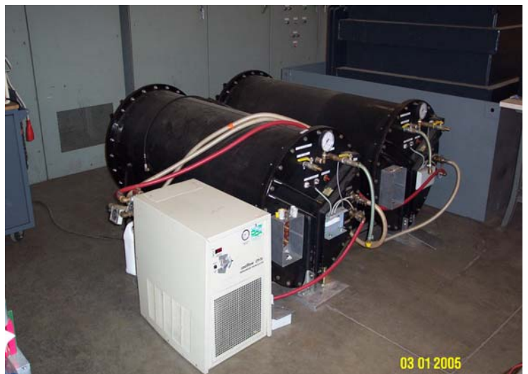
Figure 3.5: Real-time matching system showing transmission line box which also contains the ferrites and bias magnet.
