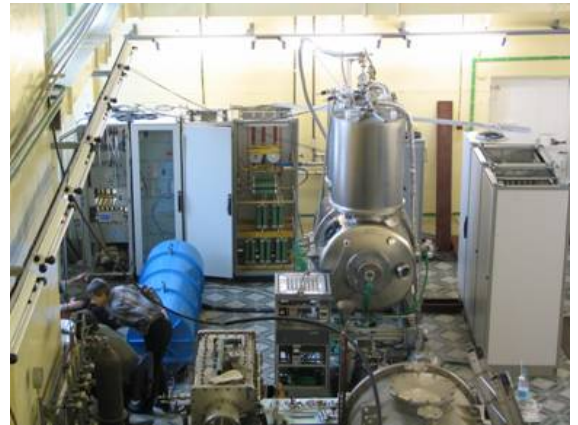
Figure 3.3: The long pulse diagnostic neutral beam undergoing testing in Russia
