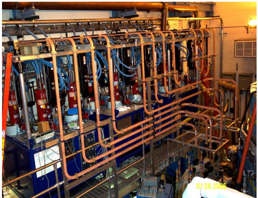
Figure 3.2: Lower hybrid klystrons and waveguides
