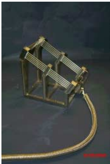
Figure 10 – Partially constructed active MHD antenna (1 of 4) for C-Mod
