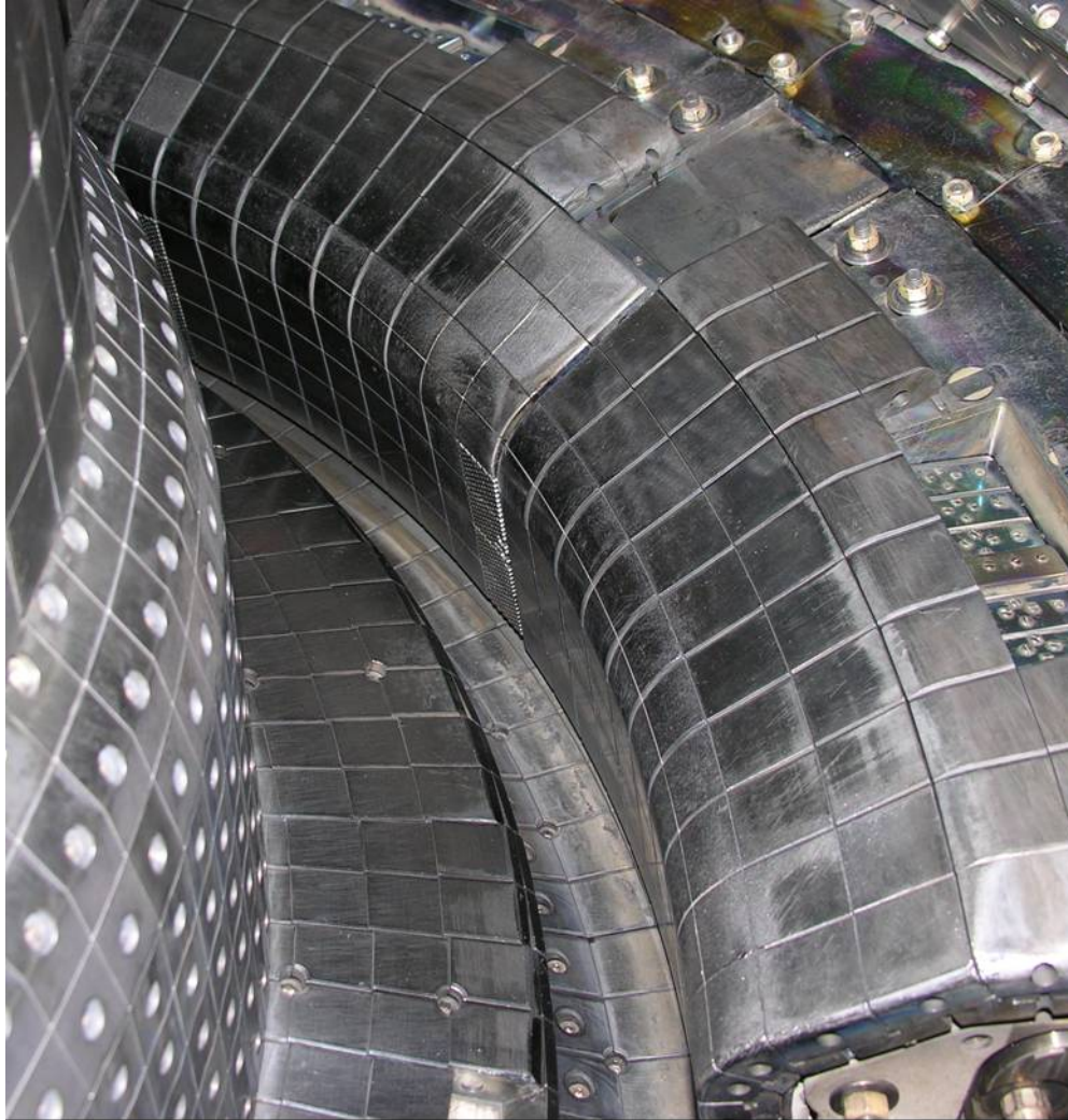
Figure 3.9 The new lamella W-tiles will form a toroidal belt just below the “nose” tiles of the outer divertor. Some of the W-brush tiles successfully tested in the FY2005 campaign can be seen near the middle of the picture.
