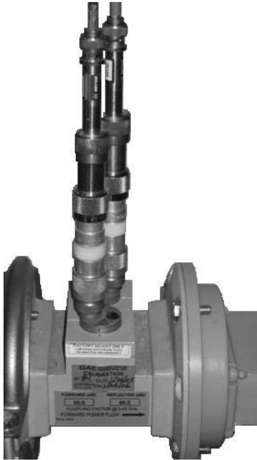
Figure 3-2: 2.45 GHz directional coupler with the DC block, attenuator, and detector diode attached.
