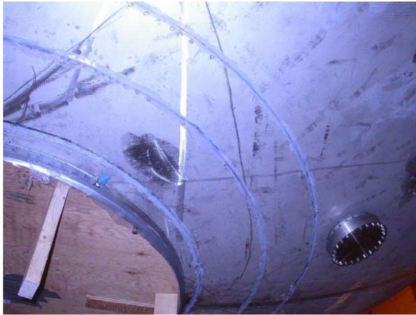
Figure 2-2: Flux loops at the bottom of the vessel.
