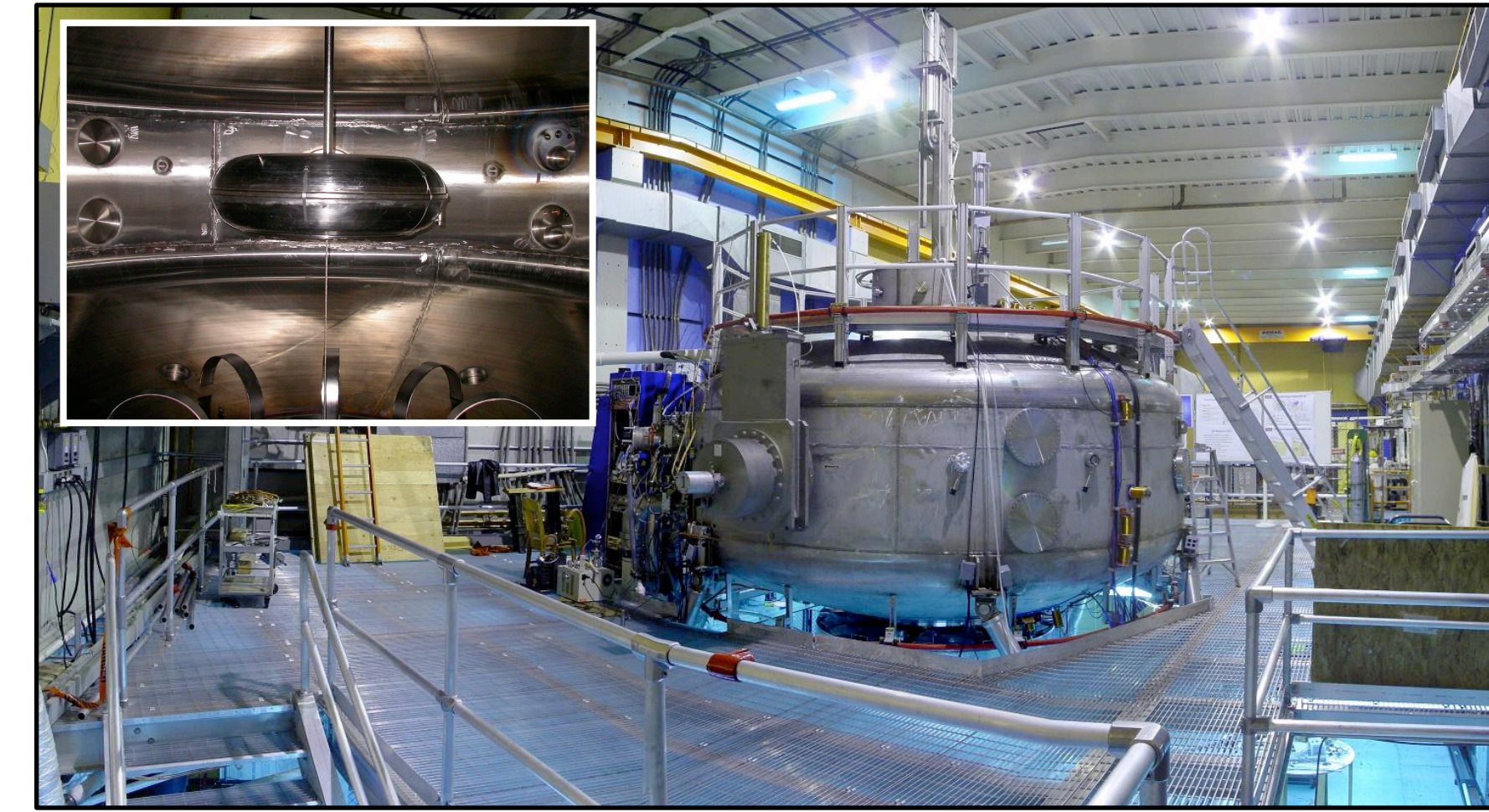
LDX experiment. The vacuum vessel is 5 m in diameter and the 560 kg superconducting dipole coil is 1.2 m in diameter.
