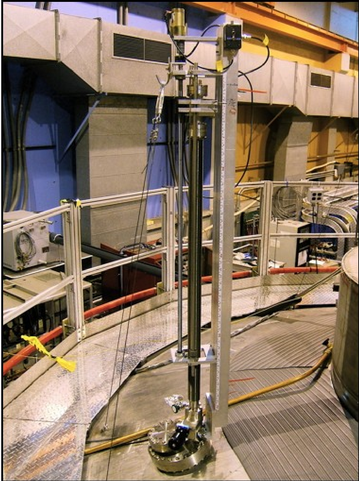
Figure 2-12: The probe motion system on LDX enables computer controlled linear motion. The stand is designed to allow in situ replacement of a probe tip without breaking the main vessel vacuum.
