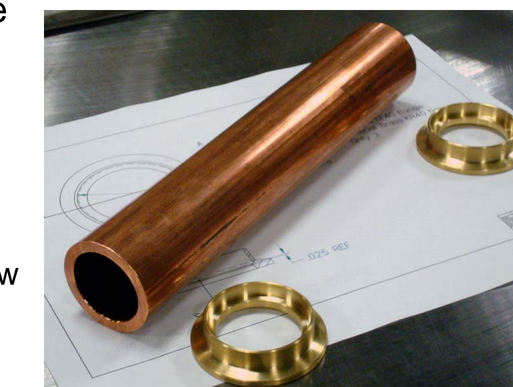
32.5 mm internal diameter and 10 mm wall copper bus bar tubing for straight waveguide run and Vlasov antenna.
