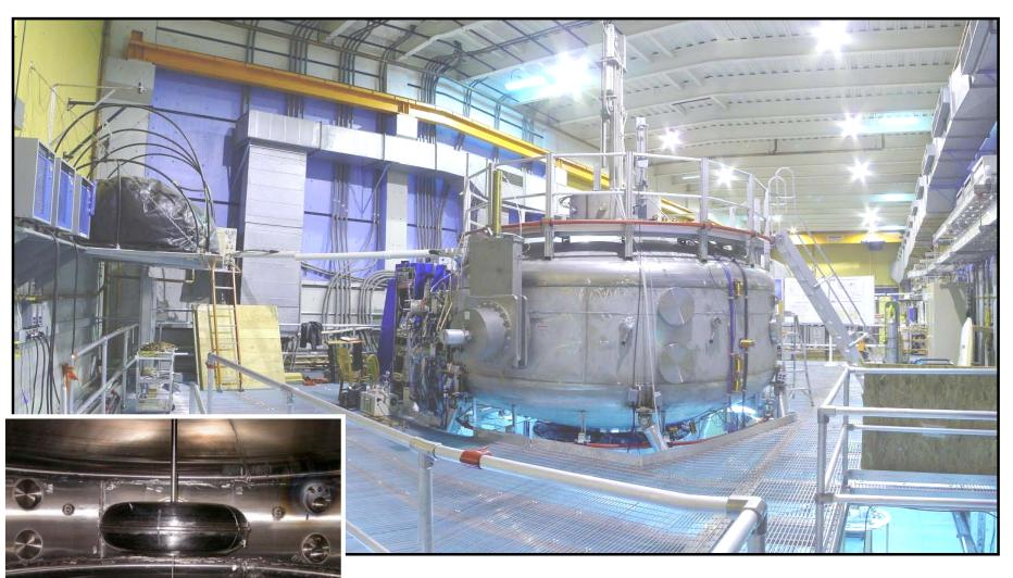
1200 lb floating coil is levitated within 5 m diameter vacuum vessel
