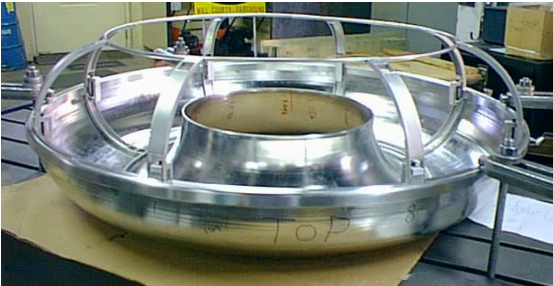
Cryostat vacuum vessel and support space frame
