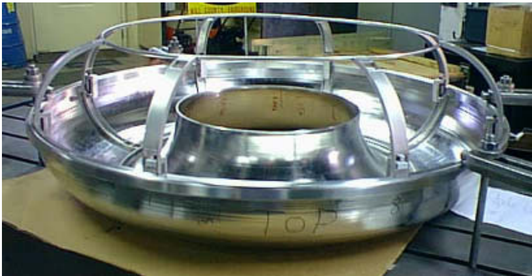
Cryostat vacuum vessel and support space frame
