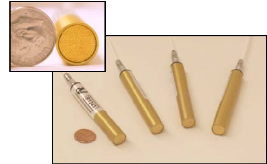
Photographs of the CZT (cadmium zinc telluride) SPEAR detectors used in the PHA.
