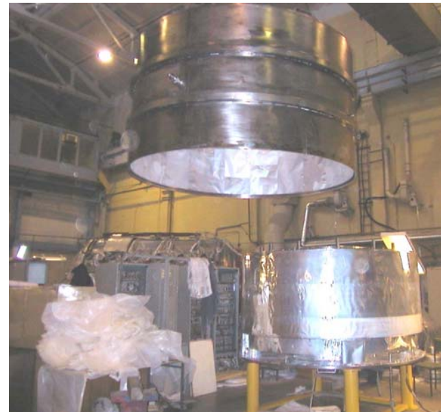
Outer vacuum vessel lowered over assembly (with outer LN2 can installed)
