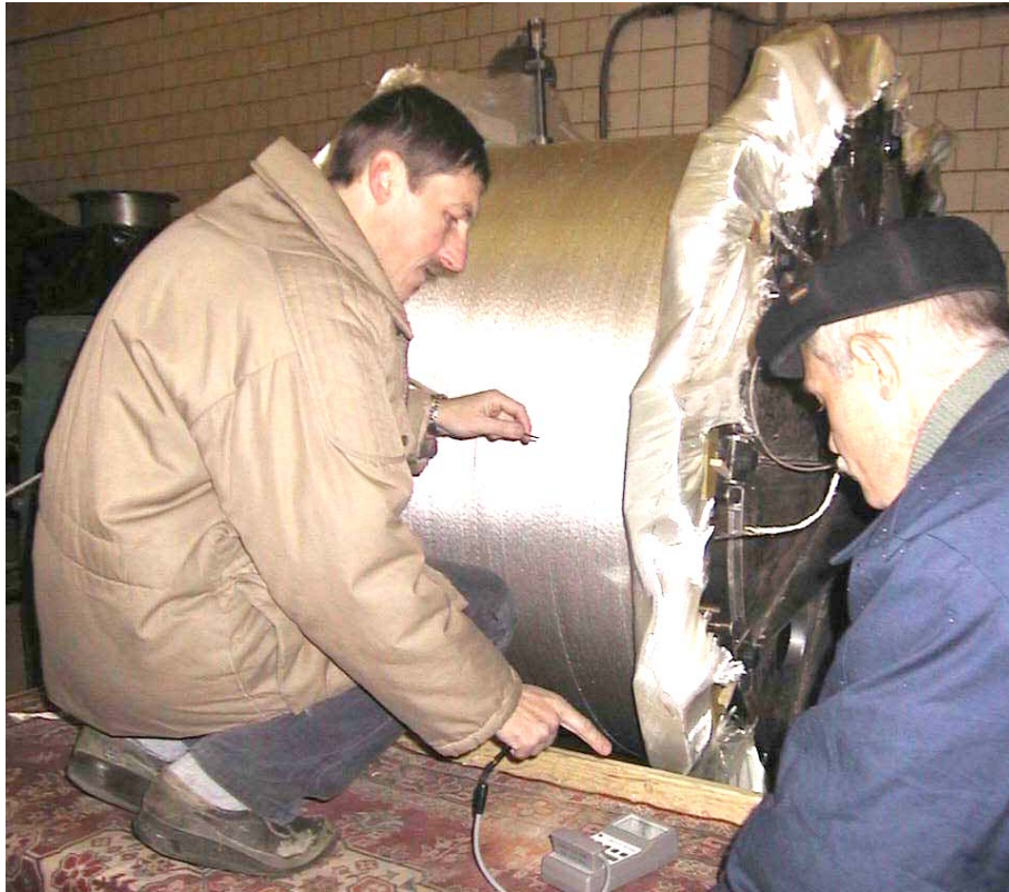
Winding 37 km of superconducting cable
