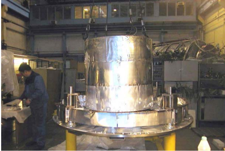
Inner LN2 can installed
