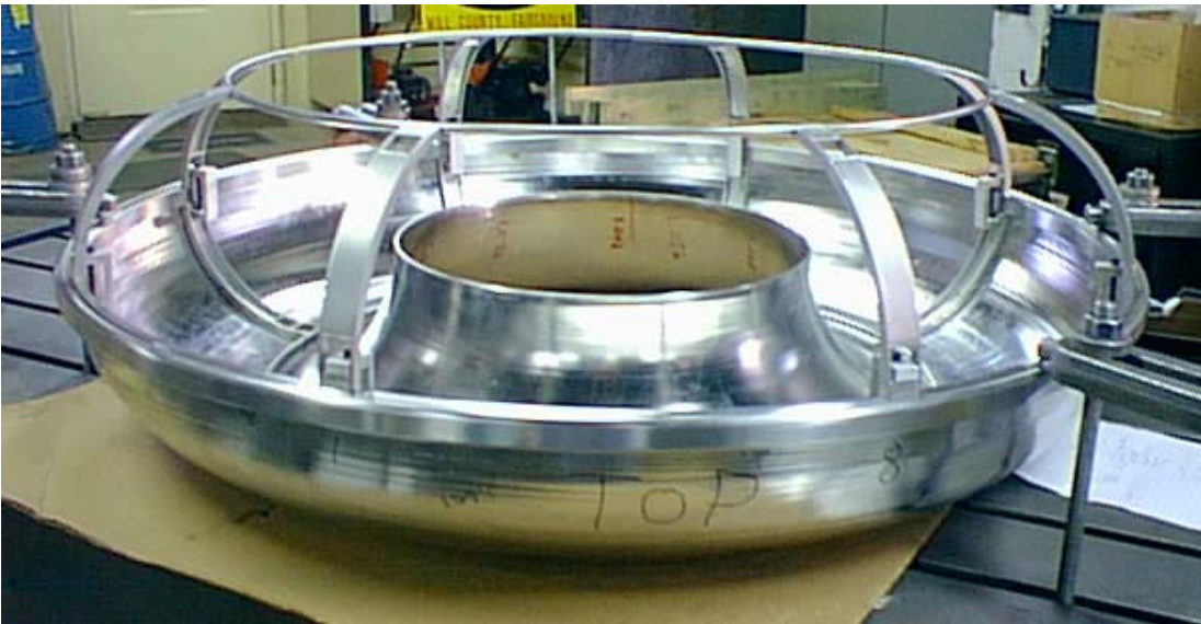
Cryostat vacuum vessel and support space frame
