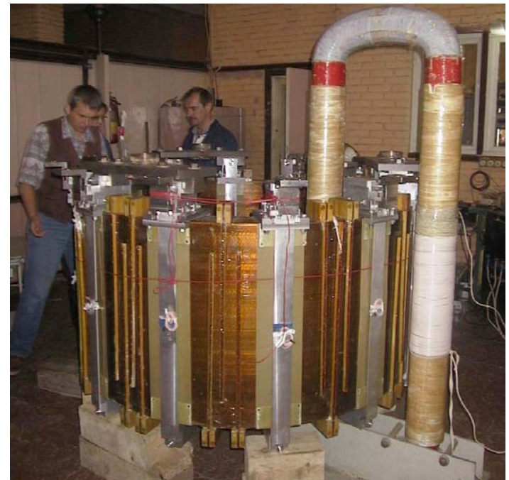
Electrical tests after 100 T of axial preload
