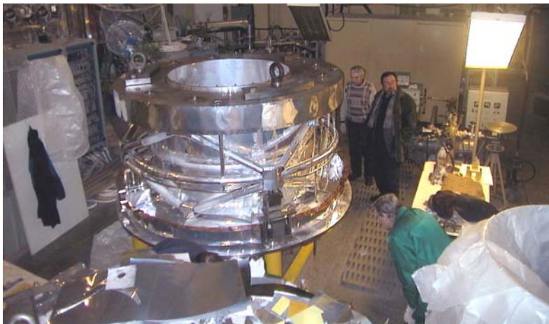
LHe can installed on LN2 cooled struts
