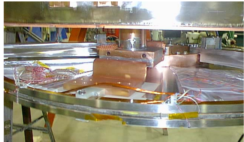
Coil in first stage of cryostat assembly
