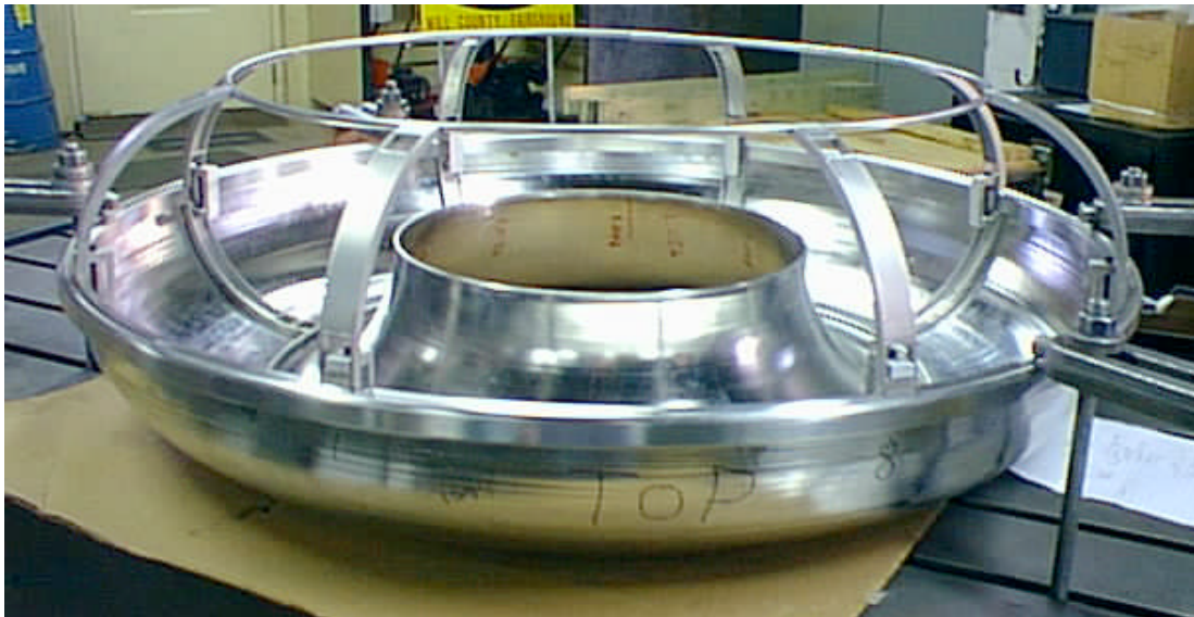
Cryostat vacuum vessel and support space frame
