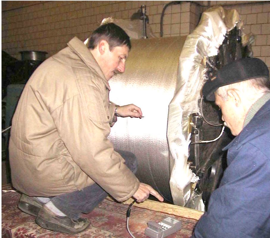
Winding 37 km of superconducting cable
