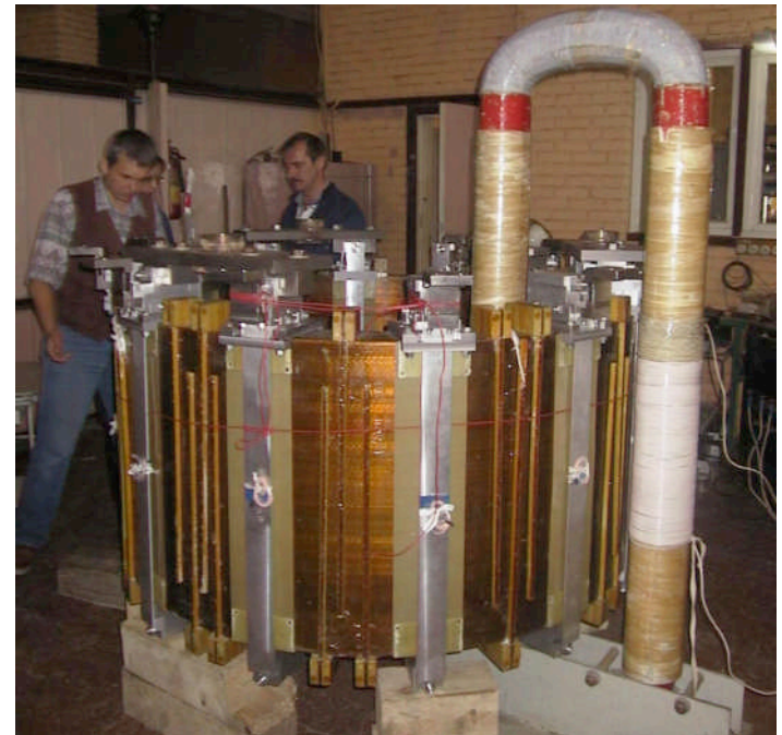
Electrical tests after 100 T of axial preload
