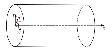
The unperturbed magnetic field has only  $\square$  component,  $B_{\square} = B_{\square 0}(r) = B_0(r)$ ;  $B_{r0} = B_{z0} = 0$ .  $\square$  and z are analogs of the poloidal and toroidal coordinates, respectively
