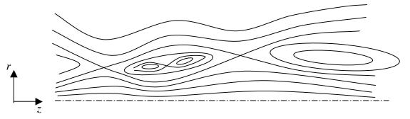
A remarkable feature of the "poloidal-field-only" systems: even an infinitesimal perturbation causes a dramatic change of the magnetic topology: without perturbations, each field line would have generated only a point on the (r,z) plane, determined by the initial z and r.
